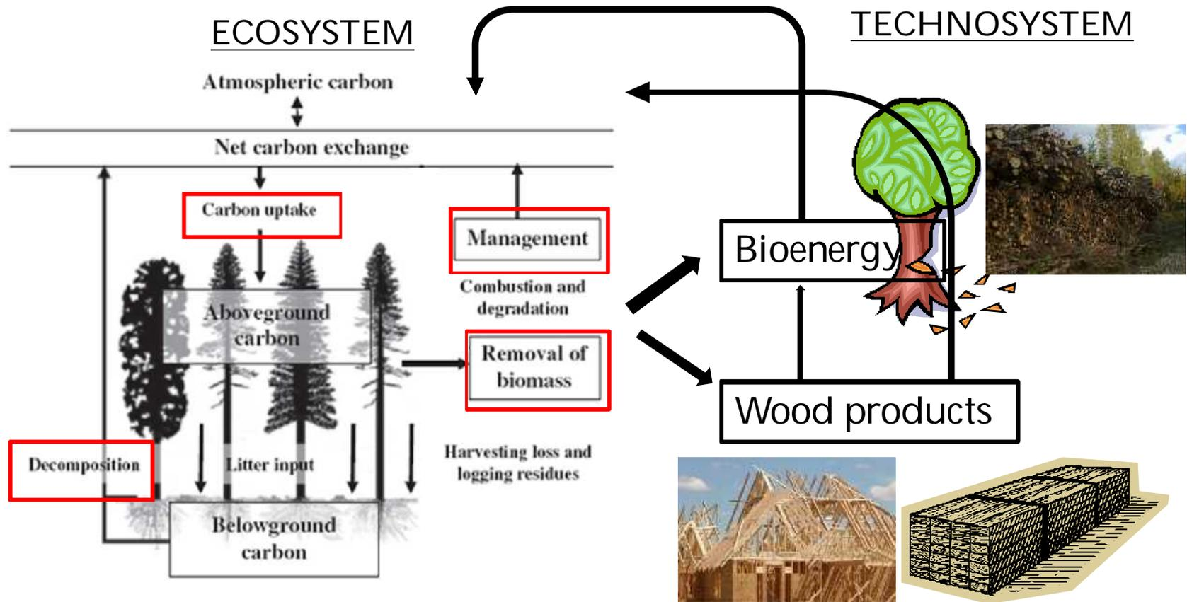
$$C_{net} = C_{seq} + C_{man} + C_{decomp} + C_{harv}$$
