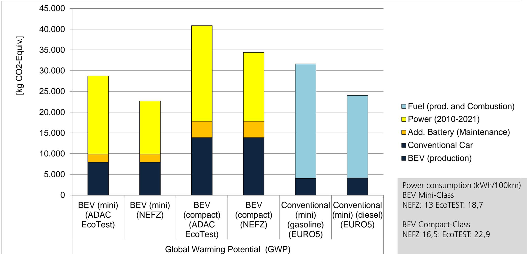
Considerable differences in the energy consumption of EVs according to chosen driving cycle, which results a variation from ~ 15 to 20% in the vehicle life cycle. The driving cycles do not necessarily reflect real vehicle specific driving profiles. These aspects have to be evaluated in future studies.
