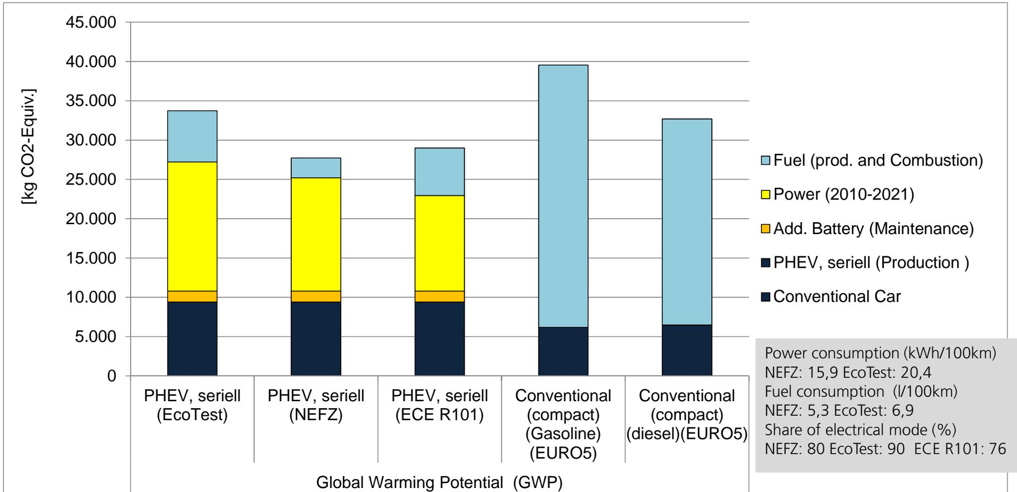
Depending on the chosen driving cycle and method for calculating the share of electrical driving mode, the results vary by ~ 16. Two methods are used: assumption by the electrical range and average driving distances (DAT report) and calculation by ECE R101. Also for the PHEVs vehicle and user specific utilization profiles are required.
